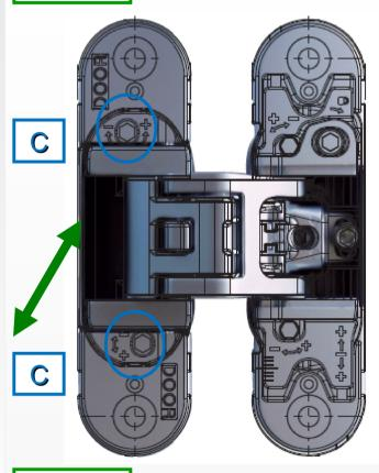
Act at the same time on screws C – Be careful: move the inner body in a uniform way
